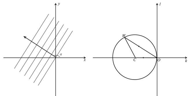
Fig. 1. Schematics for (a) a long-crested wave, slant lines are constant phase lines, and the arrow denotes the wavenumber vector,  $\alpha$  denotes the angle between the arrow and the  $x$ -axis; and (b) the circle locus of the wavenumbers in  $(k, l)$  domain for free  $\beta$ -plane waves without the basic flow, following Fig. 1 in Longuet-Higgins (1964).
