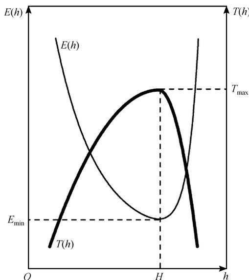
Fig. 2. Illustration of total error  $E(h)$  and effective computation time  $T(h)$  versus stepsize  $h$ .  $H$  denotes the optimal stepsize,  $E_{\min}$  the minimum error and  $T_{\max}$  the maximum ECT.
