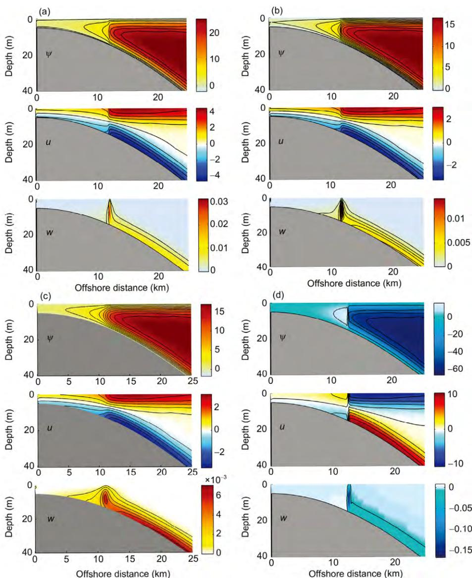
Figure 5 Streamfunction, cross-shelf velocity and vertical velocity fields for  $u_\infty = -0.06 \text{ m s}^{-1}$ . (a)–(d) correspond to stratifications 1–4 respectively. The units of  $u$  and  $w$  are  $\text{m s}^{-1}$ .
