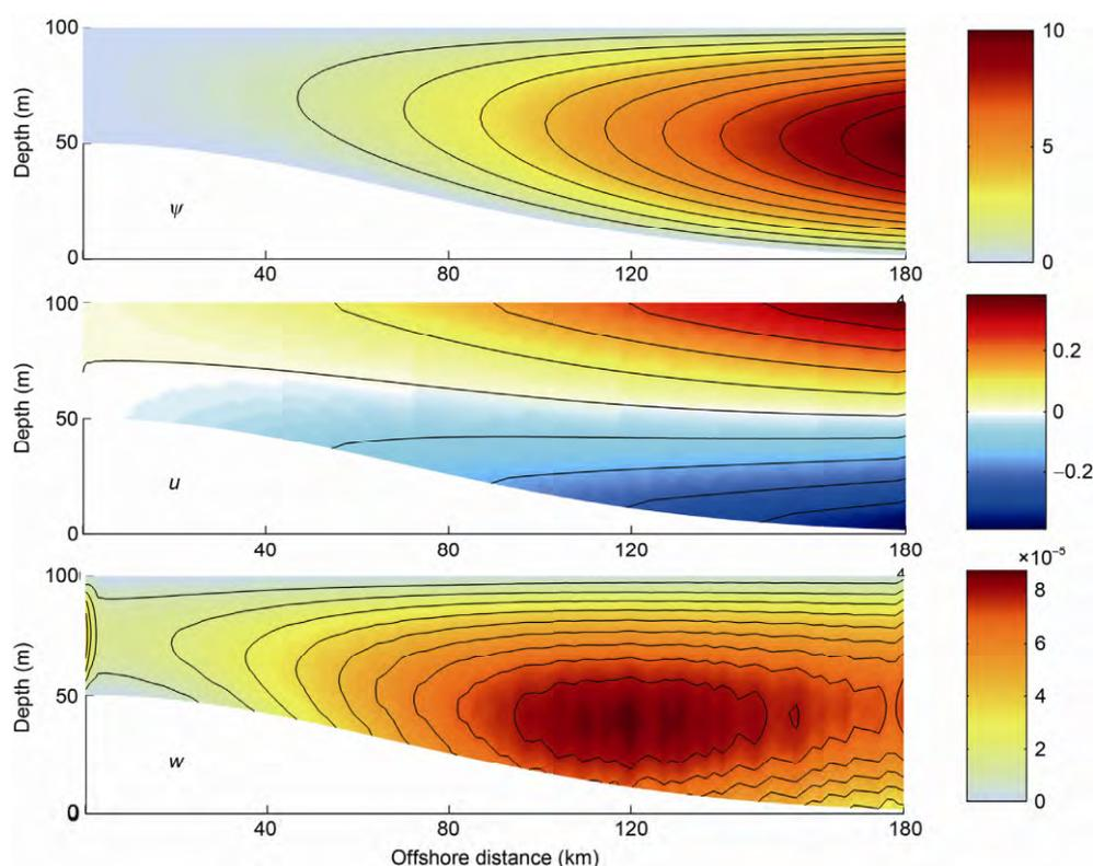
**Figure 6** Streamfunction, cross-shelf velocity and vertical velocity fields been obtained with the FEM. The units of  $u$  and  $w$  are  $\text{m s}^{-1}$
