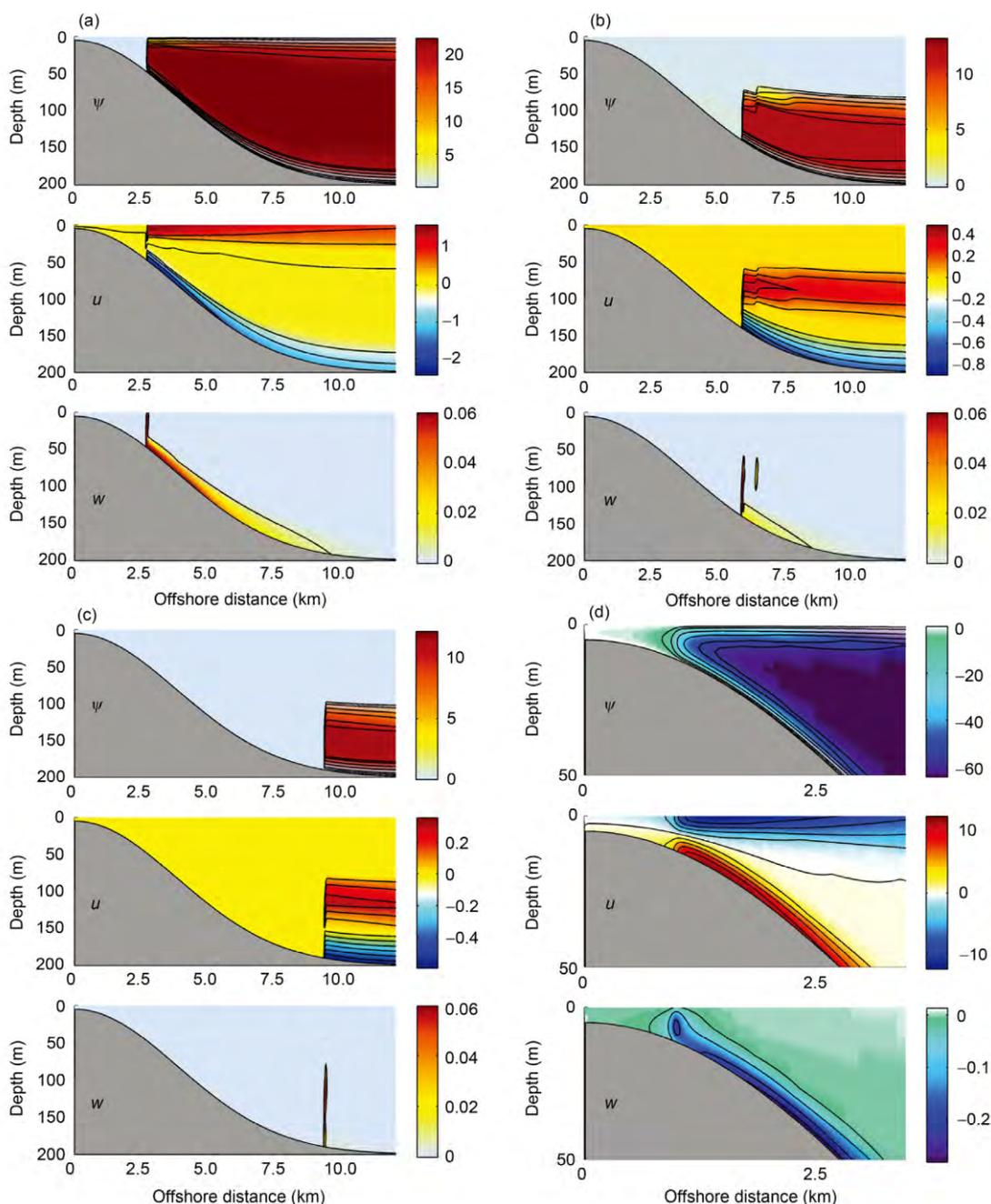
**Figure 9** Streamfunction, cross-shelf velocity and vertical velocity fields over the deeper continental shelf (depth of 200 m, offshore distance of 13 km) for  $u_{co} = -0.06 \text{ m s}^{-1}$ . (a)–(d) correspond to stratifications 1–4 respectively. The units of  $u$  and  $w$  are  $\text{m s}^{-1}$ .
